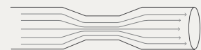
Drawing of a constriction in the pipe through which airflow is circulating.
