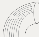
Drawing of a 90° circular bend through which airflow is circulating.
